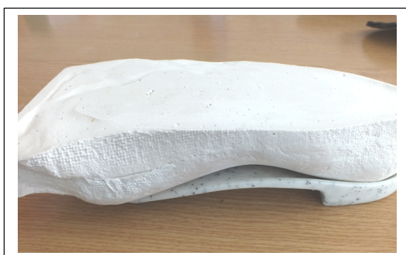
Fig 8 Pronatory imbalance due to software defaulting to a lower arch setting.
